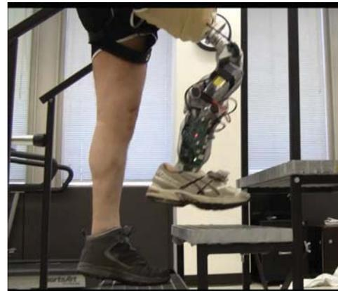
Figure 1: Vanderbilt's powered prosthetic knee/ankle device during stair ascent.
