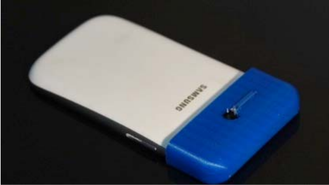
eFigure 1. Peek Retina 3-Dimensional Printed Prototype Adapter Fitted on a Samsung SIII Smartphone
